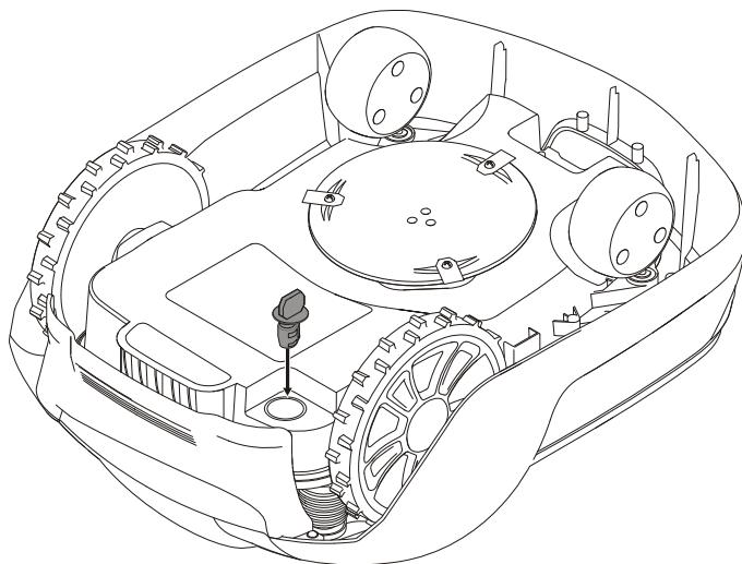
Insert the safety key into the underside of mower and turn to the **Enable** position.
