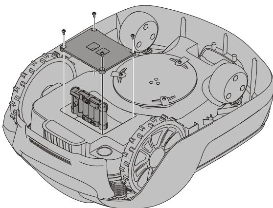
**WARNING!** Press the STOP button and remove the safety key before replacing batteries and wear protective gloves.
