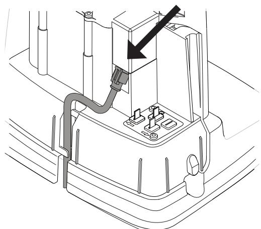
Connect the low voltage cable to the charging station.
