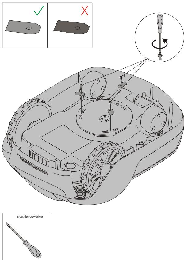
**WARNING!** Press the STOP button and remove the safety key before replacing blades and wear protective gloves.
